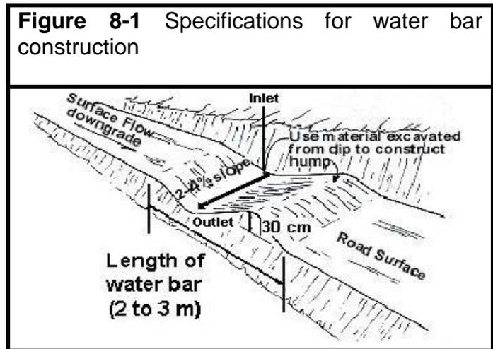
Extend the inlet end of the water bar swale to the invert of the roadside ditch to intercept all the runoff.
