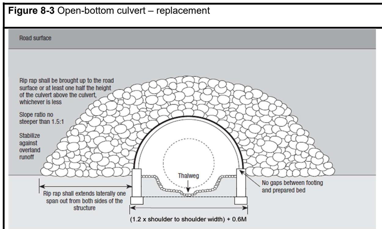
The reconstructed channel must be restored to its natural grades and to the cross-section immediately upstream and downstream of the altered area (*i.e.* a reference reach outside of the impacted zone). See Figure 8-3.
